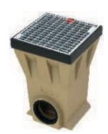
The yard gully is made from polymer concrete. It has a superimposed cast frame, an internally located cast frame or a grating made from galvanized steel mesh and it is fixed with the Pointlock system of screwless locking devices.
