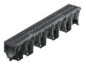
The ACO XtraDrain drainage channel has a plastic composite grating. It is permanently resistant to corrosion and it is a visually attractive unit in the B 125 loading class.
