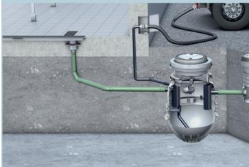
Standard: All ACO Grease separators are manufactured in accordance
